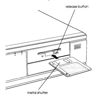
To insert a diskette into a 5.25-inch drive, hold the diskette with the label facing up and the read/write slot leading into the drive. When you want to remove the diskette, make sure the drive light is off; then press the release button or flip up the latch. When the diskette pops out, remove it and store it properly.
